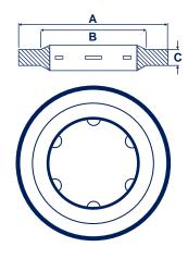
A nylon captive sealing washer for screwed assemblies, suitable for applications of 200 lbf/in² working pressure.
