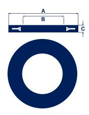
A dual purpose, vibration resistive lock washer, which protects as it locks. Ideal for surface coated with paint, plating, enamel, etc. Suitable for use with water, mineral base oils and alkalis, over a temperature range of -10°C to +80°C. Extensively used in the automotive and domestic appliance industries.
